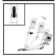
Press the **Flexology\* Wand Unlock Latch** on the back of the wand then adjust the angle.
