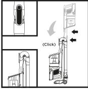
To put the vacuum into storage mode, press the Flexology wand unlock button while folding the handheld vacuum forward until it is resting against the wand.
