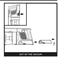
To remove the battery from vacuum, press the release button on the battery and slide out handle compartment. To reinstall, slide the Battery back into the compartment until it clicks into place.
