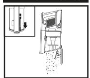
To empty the Dust Cup while it is attached to the handheld vacuum, position the dust cup over a dust bin and slide the Lid Release slider forward.
