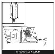
Remove the handheld vacuum from the wand by pressing the **Wand Release** button and pulling up. Plug the charger into the charging port on the handheld vacuum.
